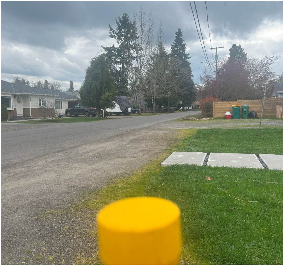
Figure 5: Available Sight Distance Looking South at 14.5 feet from Edge of Travel Lane
